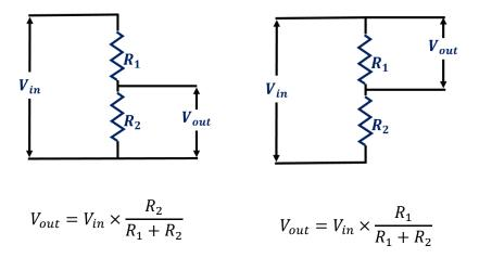
A general rule that can be applied for any voltage divider circuit is as follows:
